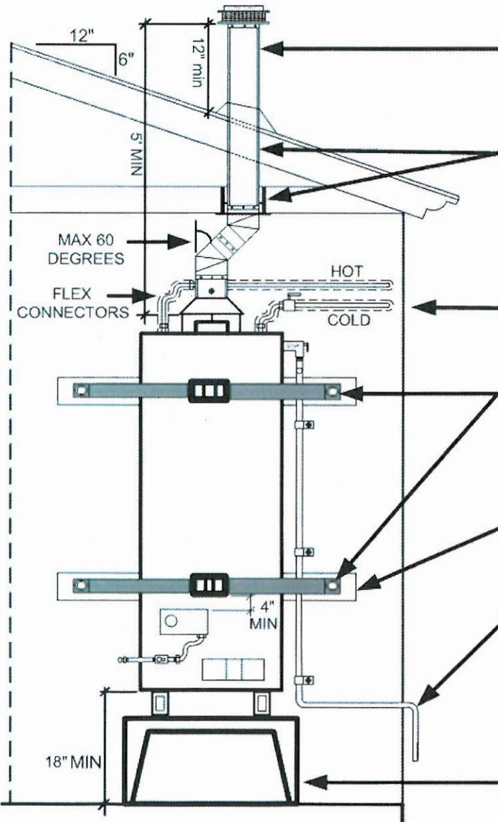
Venting for the water heater shall be Type B (double wall) vent pipe and shall terminate at least 5 feet above the draft hood or flue collar and at least 12" above roof. (steeper pitched roofs will require additional clearances)
